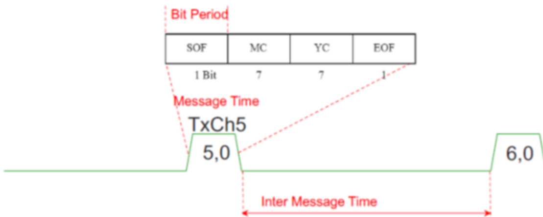
FIGURE 9-1 ILLUSTRATION OF MESSAGE AND INTER-MESSAGE TIMING
